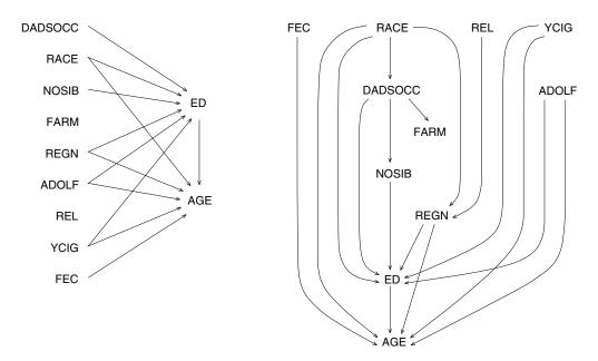
Given the prior information that ED and AGE are not causes of the other variables, the PC algorithm (using the .05 significance level for tests) directly finds the model [in the left hand panel of Figure 8] where connections among the regressors are not pictured. [1993, p. 139; 2000, p. 103]
